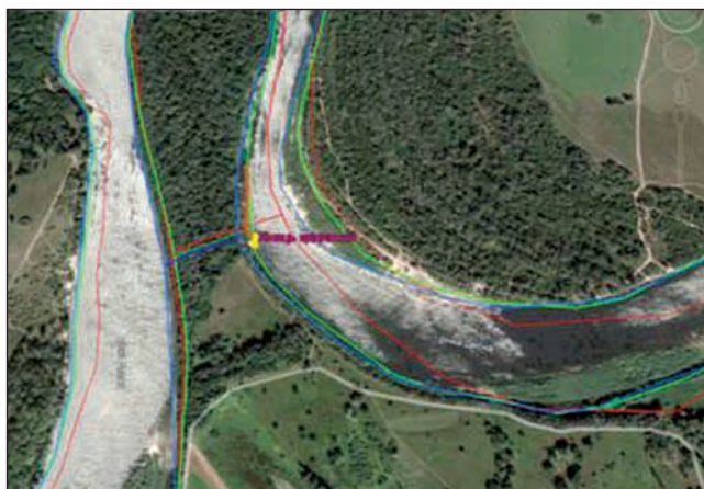
Fig. 12. Combined contours of the left bank of the meander in the section of the land bridge
